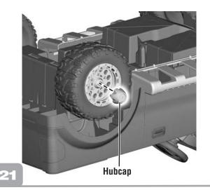
• Align the tabs on a hubcap with the slots in a rear wheel. "**Snap**" a hubcap into the center of the rear wheel.
